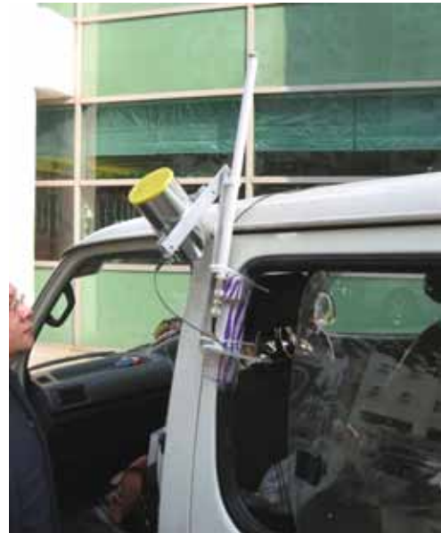
Figure 3: The two antennas mounted on a site-surveying mobile-testing van. The circular one is the waveguide antenna and the tube-like one is the collinear antenna built by students. The vehicle used is the same van used in testing Hong Kong's 3G mobile station, which was commissioned by Hutchison Global Communications.
